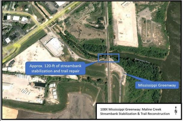
The project design was added to the Capital Budget for 2023 under project #108X. The images below highlight the downstream bank and greenway trail adjacent to the railroad bridge that has been failing more steadily into the creek since July. The undercut has caused the trail pavement to collapse and created a tight pinch point for the trail.
